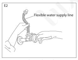
E2. Use Wrench to tighten the water supply hoses, please do not overtighten the connections.
