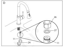
D. Install counter weight (24) onto pull out hose (11). Connect the pull out hose to water inlet tube (26). Be sure to install rubber washer (27). Do not overtighten the connection.
