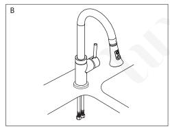
B. Place flange (19) and washer (20) under the new faucet. The faucet hole on the mounting surface should be 1 1/2" in diameter.
