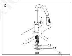
C. From under the sink, install the black rubber washer (21), metal washer (22) and nuts (23) onto the mounting tube (29) Tighten the nuts to secure the faucet to the mounting surface.
